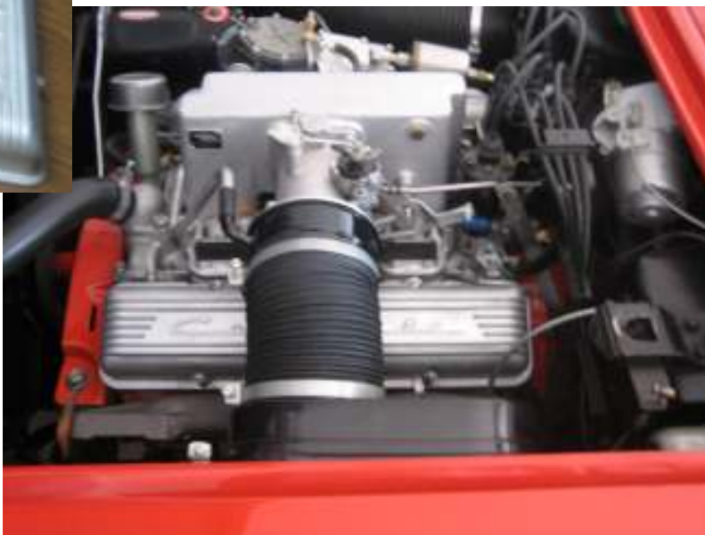
Picture of 1960 7320 that was reassembled after refinishing and installed on my 59 for calibration and road test .This unit runs real well and is now ready to ship..
