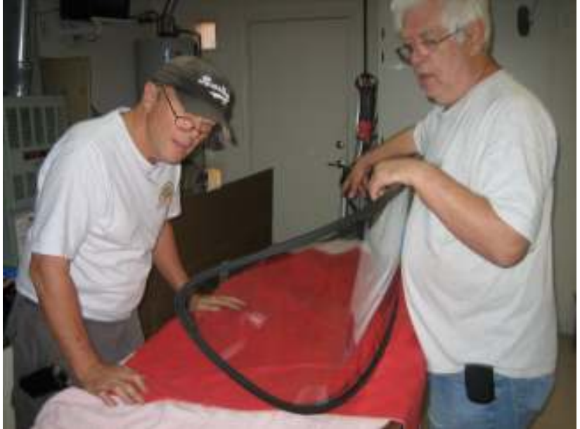
Garry and Mike checking windshield gasket location - note the mark placed on the glass to insure that the flat part of the gasket will lay slightly over the post.
