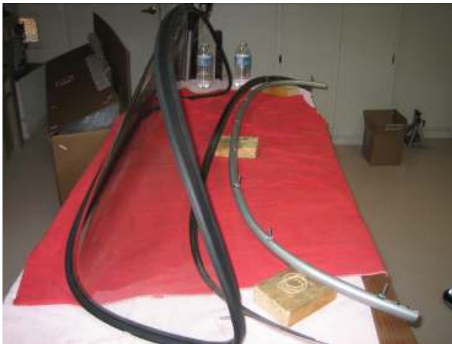
Picture of lower channel and stainless trim . Show the T bolts and the anchor slots where the anchor plates will be held in place with strip calk. Channel and trim must be installed as a unit.
